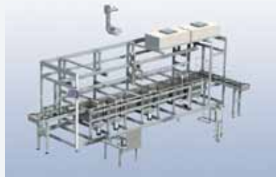
Ultrasonic cleaning lines composed of modular components
